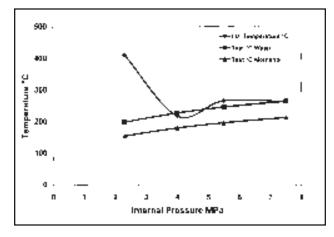
Fig. 3 — Pipe inside wall temperature for 50% methanol in water (1.45 kJ/mm) and T<sub>sat</sub> (methanol and water) vs. pressure.
