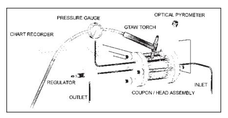
Fig. 1 — Pressurized pipe test assembly.
