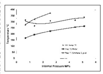
Fig. 5 — Pipe inside wall temperature for 50% ethylene glycol in water (2.0 kJ/mm) and  $T_{sat}$  (water and ethylene glycol) vs. pressure.
