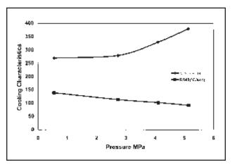
Fig. 8 — Outside wall cooling rates for 50% ethylene glycol in water (1.4kJ /mm).
